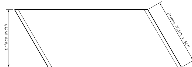
PLAN OF SUPERSTRUCTURE SLAB
